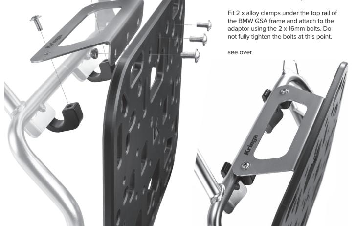
3. Fit the remaining 4 x alloy clamps in the positions as illustrated below.
